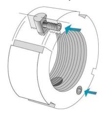
These instructions are meant to ensure that the gibs are correctly tightened by means of eccentric screws.
